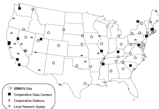
Figure 1. Existing and planned USNSN telemetry sites projected for the fall of 1992. Note that the octagons and triangles represent broadband stations while the diamonds show RSN sub-network nodes and the squares show cooperating data centers.
